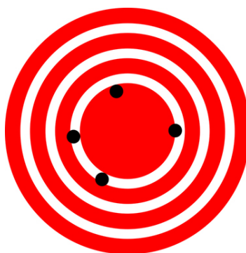
Figure 1.24 A GPS system attempts to locate a restaurant at the center of the bull's-eye. The black dots represent each attempt to pinpoint the location of the restaurant. The dots are spread out quite far apart from one another, indicating low precision, but they are each rather close to the actual location of the restaurant, indicating high accuracy. (credit: Dark Evil)
